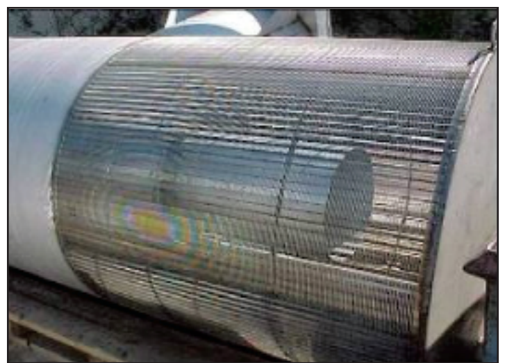
Figure 7. Wedgewire Ocean Intake Structure (Photo courtesy of West Basin Municipal Water District)
